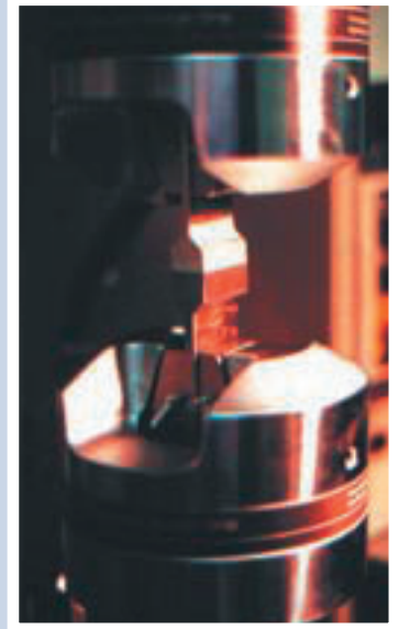
Through thickness tensile test of Triplate
